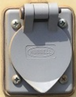
Power Inlet 15 Amp Battery Charger
