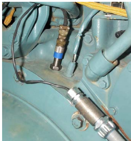
Illustration 12 - MPU, Strain Relief and Sealrite
