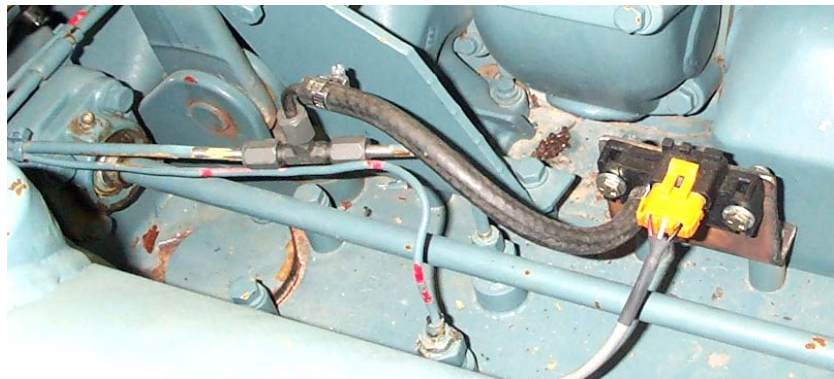
MAP Mounting on Intake Manifold
